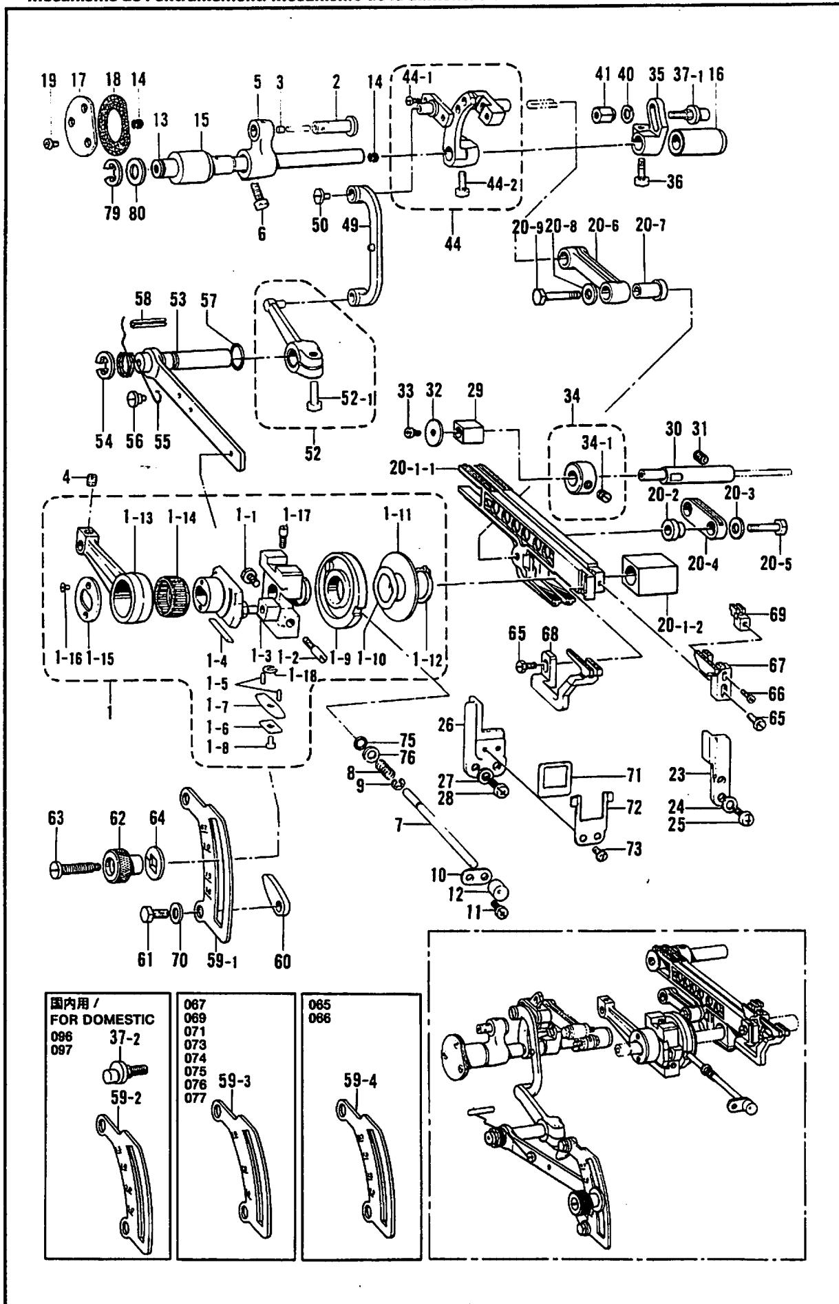
F. 送り関係/Feed mechanism/Transportvorrichtung/
