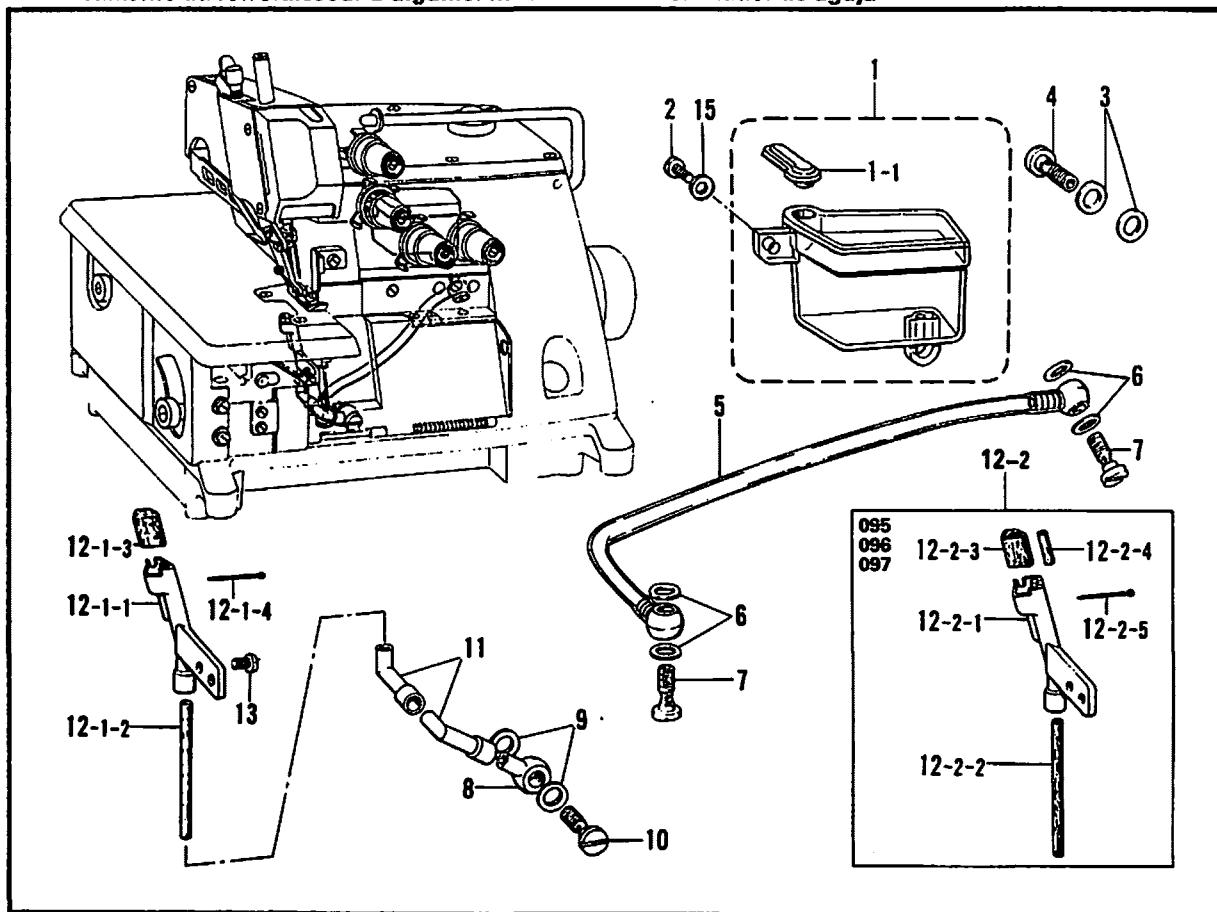
B. 駆動軸関係/Crank shaft mechanism/Kurbelwelle/
